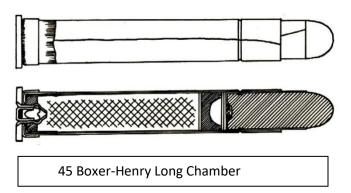
Competition was opened to anyone wanting to submit a new rifle and cartridge. The rifle that was chosen was the Martini-Henry and the new cartridge was the Boxer-Henry. This cartridge was 45 caliber and had a straight coiled built-up case that was 3.220" long and had a base diameter of .555". The overall length of the cartridge was 3.750". This long cartridge was not satisfactory although improvements to it did make it better.
