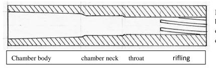
Modern rifle chamber for metal jacketed or lead bullets. The throat keeps the bullet from contacting the rifling when the round is chambered.
