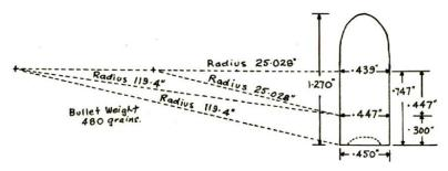
The bullet was paper patched with the patch being applied left to right. If the bullet is held with the base toward the person the leading edge of the outer wrap will be to the left of the bullet. Two wraps were used. The patch was twisted into a tail and pressed into a hollow in the base of the bullet.
