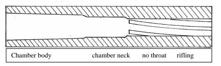
Chamber made for paper patched bullets. There is no throat and the bullet slips into the barrel and rests on the rifling.
