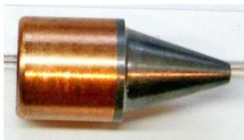
Conical point bullets are sometimes used for handguns. If used in a rifle and with a longer point the bullet would be called a spire point. This one has an 18 degree angle which makes it somewhat long for handgun use. A wider angle and shorter nose would be more common. But once again it is up to the bullet designer and no single design.
