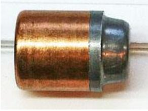
Another semi-wadcutter style that is popular is the H&G 68 Short. This design has the corners of the bullet's nose more rounded in order to improve feeding when used in autoloading handguns. It is a good short to medium range design and would be an effective defense or hunting bullet. Like most SWC types of bullet it could be made with or without a hollow point.
