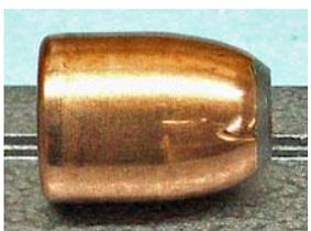
This is a fully jacketed bullet which is often incorrectly called an FMJ or Full Metal Jacket. This bullet has the jacket cover most of the ogive leaving the front of the bullet open. The bullet can have a hollow point, or an open tip, or a solid lead tip. The amount of lead exposed at the front of the bullet can vary but always the ogive will be covered by the jacket enough to prevent leading of the gun bore. The base of the bullet is covered by the jacket. The base can be flat or cupped.
