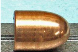
The FMJ or Full Metal Jacket bullet has the ogive completely covered by the jacket. There is no exposed lead, no opening at the front of the bullet, and by design the bullet is not expanding. The base of the bullet is open and the core is exposed. Generally the bullet jacket is rolled over and flattened to prevent the jacket from being blown apart by the muzzle blast as the bullet leaves the barrel. This type of
