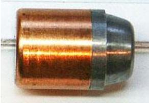
This is a semi-wadcutter style that has a round nose flat tip. A round nose like a 3/4E ogive is cut off to make a flat tip. The flat tip very much improves the bullet performance for hunting or defense. The rounded profile of the bullet with rounded corners at the flat tip improves feeding. The shape of the round nose can be anything wanted as there is no single round nose design.
