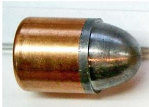
This is a 3/4E round nose semi-wadcutter. The name, 3/4E, doesn't mean much of anything but it does indicate the ogive length. The length of the nose would be three quarters of one caliber. In this case the bullet has a diameter of .452" making the length of the nose .339" more or less. The round nose is a less effective defense or game bullet than a flat tipped bullet but it is a common style.
