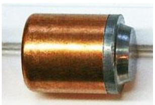
This is a semi-wadcutter that has a short nose. It is often called a button nose. The nose shape can be anything that is wanted from a very short round nose to the short truncated conical shown here. The bullet is usually used for light, short range loads and is a good choice for paper punching at fifty yards or less. The bullet in the photo would be considered a three quarter jacketed bullet as the bearing of the bullet is almost completely covered by the jacket.
