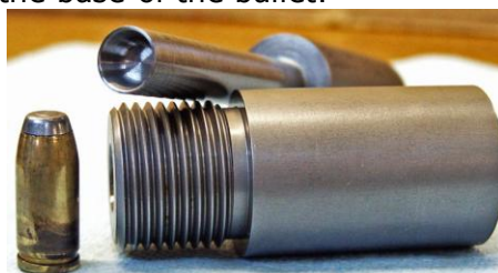
Lead tip die and internal punch. The cavity in the punch reshapes the soft point on the bullet.
