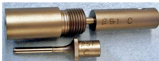
Core seat die & punches. The die and internal punch are marked with the bullet diameter and the letter C for core seat. The seating punch is marked the same and with the diameter of the punch tip.
