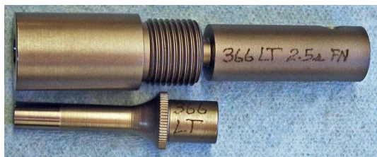
Lead tip die & punches. The die and external punch are marked with the bullet diameter and the letter L, sometime LT. The internal punch is marked the same and also with the ogive of the bullet.
