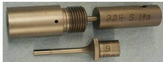
Core swage die & punches. The punches and dies are marked with the caliber, S for core swage, and the diameter of the core made. Note the bleed hole in the side of the die.
