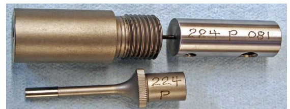
Point form die & punches. The die and punches are marked with the bullet diameter , the letter P for point form, and the ejection punch is also marked with the ejection pin diameter.
