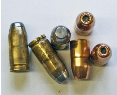
9.3 mm bullets made using commercial jackets and fired CF case jackets. Note the two diameter bearing of the bullets.
