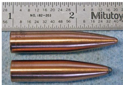
.338 bullets made with tubing jackets. Lead tip & tight open tip.
